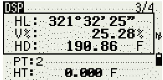
Press **DSP** to see the fourth BMS screen. This screen is the most useful when using the EDM features of the total station, comparable to the first screen when used as a theodolite.
