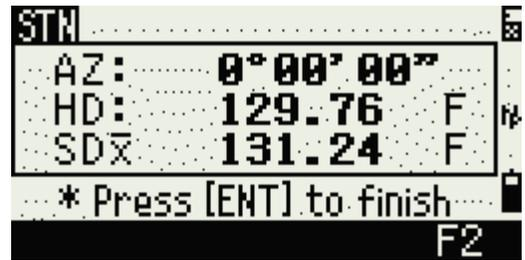
The total station is now ready to measure and record points, referenced to a known grid with a known orientation. It is now possible to dismantle the instrument and re-install it at this point, and knowing the BS, be able to re-establish the total station relative to this grid in three dimensions.
