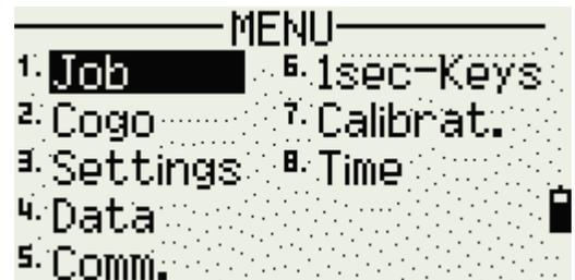
Scrolling to the Job function and pressing **REC/ENT** or pressing **1** will bring up the Job Manager window. Note the "soft keys" (Creat, DEL, Ctrl, Info) at the bottom of the LCD display.
