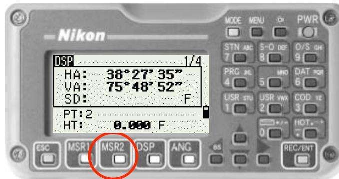
MSR1 and MSR2 can each be set up as prism-less or prism based measurements. We have set MSR2 up as prism-less. Press **MSR2**
