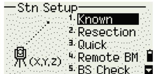
For the initial station set-up we will use option 1, **Known**. When re-establishing the location of a total station on an existing coordinate grid it is preferred to set up over previously established
