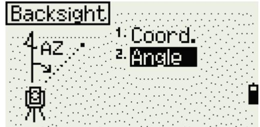
If we were using a point known to the total station we would enter that point's number on the line for BS. It is not necessary for this to be a point with known coordinates, only one that we can find again to re-establish the grid orientation. This being the case, we do not have to identify the BS and can skip by this entry by pressing the **REC/ENT**, key.
