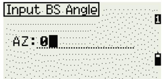
This brings up the screen which sets the orientation of the 0° horizontal angle. The BS point that has been chosen is sighted through the telescope and the **MSR** key which corresponds to the type of reflector being sighted (reflector or reflector-less) is pressed.
