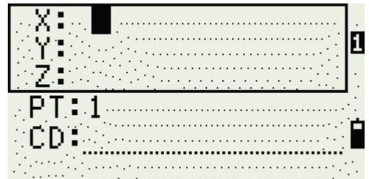
At this time we are not covering the use of point codes (the CD entry), therefore this line can be left blank. Pressing **REC/ENT** brings back the Input Station screen
