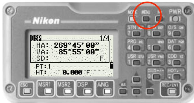
The first step is to create a "job", which is basically a data file with specific settings pre-selected as discussed earlier. The Job function is accessed through the Menu which is reached by pressing the **MENU** key.
