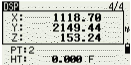
Recording the information about a point is also straightforward. Pressing **REC/ENT** after measuring a point automatically records the data and brings up a blank entry screen for taking the next point's measurement data
