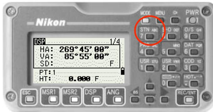
Access the Stn Setup menu by pressing the **STN** (7) key while in the BMS screen. In the Stn Setup menu there are seven choices to pick from; to see the final two you have to scroll through the menu items until you reach the second screen.
