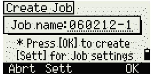
Pressing the **ANG** key, which corresponds to the **OK** soft key finishes the process of the job creation and returns back to the BMS.
